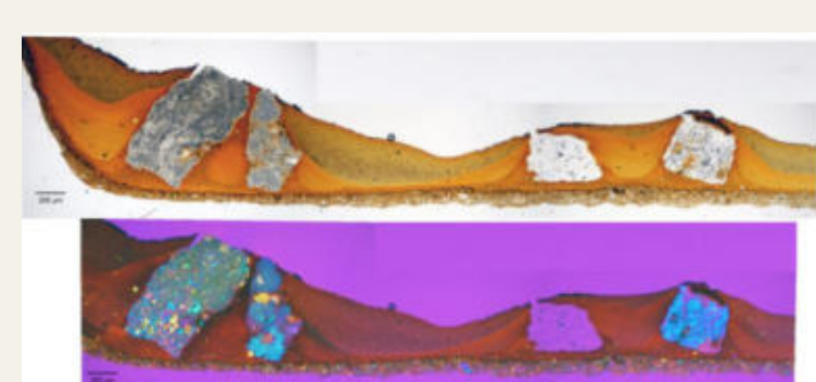
Fig. 5. Cross section image of the protrusion part: a) transmission image, b) polarized image.
