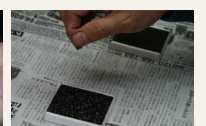
f. Sprinkling the stones on the still wet lacquer surface. Type A, B.
