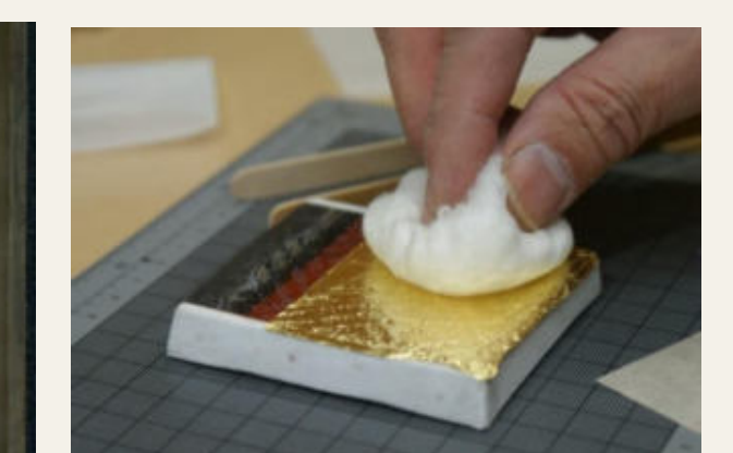
l. Application of gold leaf with. Type A, B.
