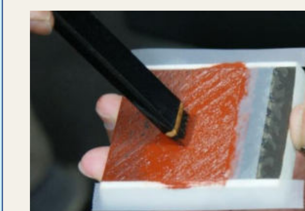
j. Application of red urushi shu-urushi . Type A, B.
