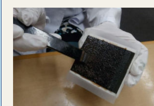
g. Fixing the pattern with kijoumi-urushi . Type A, B.
