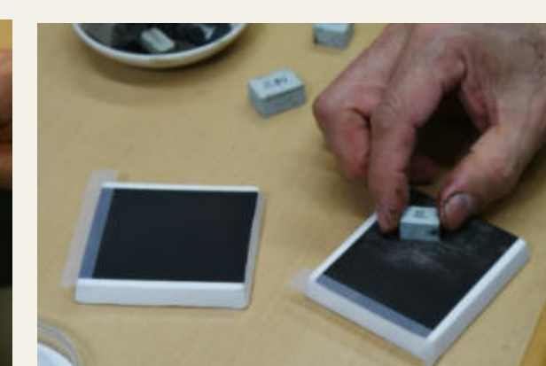
b. Polishing the foundation surface. Type A, B.
