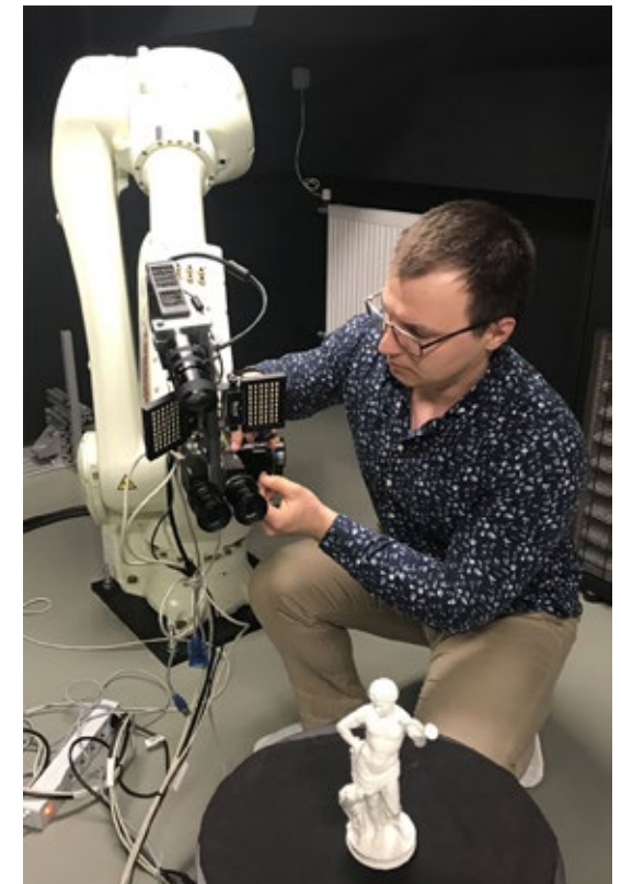
Setting up structured light scanning equipment, photo E. Bunsch
